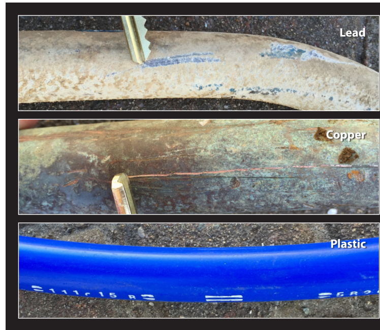
Most residential water service lines in Concord are made of Lead, Copper or Plastic. Lead service lines are generally a dull gray color and are very soft. You can identify them easily by carefully scratching with a key. If the pipe is made of lead, the area you've scratched will turn a bright silver color.
