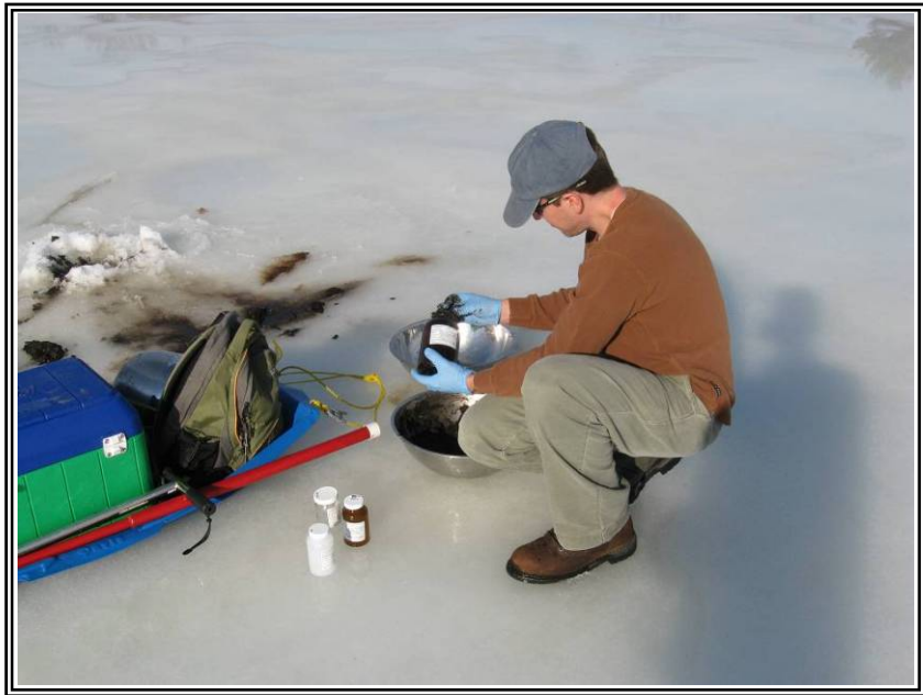
Photograph No. 6: Mixing composite sample and collecting in lab jar
