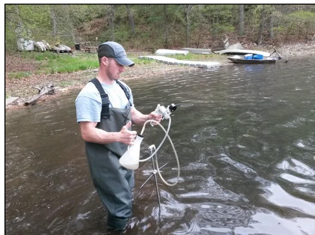
Collection of shallow groundwater with a littoral interstitial porewater sampler.
