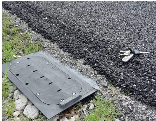
Example of GKY FirstFlush sampler installed for collection of road runoff.
