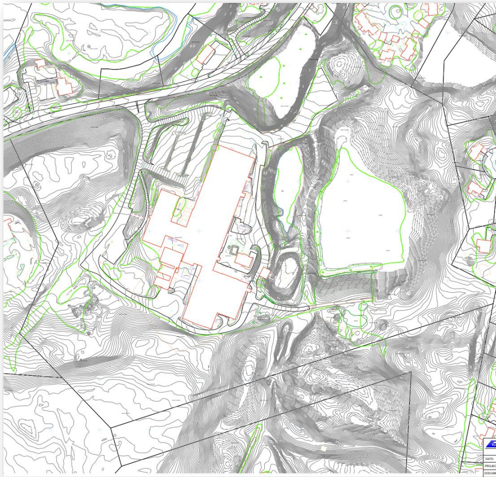
FIGURE 4.1. Topography of the site. Notice flat areas (white patches) include the building foundation dominating the eastern portion of the site and wetlands/ponds/bogs separated by steep banks (black lines close together) dominating the western half of the site.
