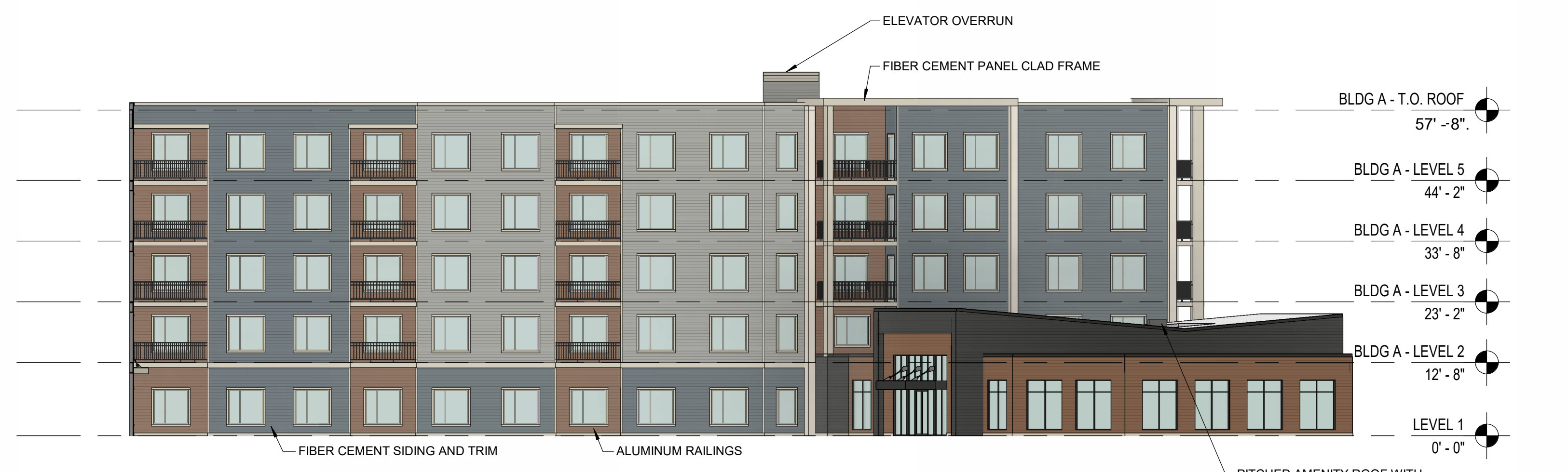
04 BUILDING A COURTYARD ELEVATION - SOUTH Scale: 1/16" = 1'-0"
