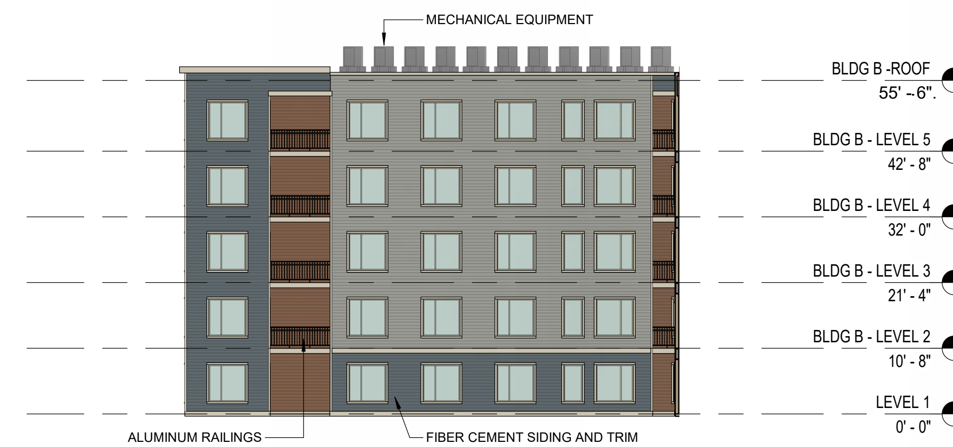
05 BUILDING B COURTYARD ELEVATION - NORTH Scale: 1/16" = 1'-0"
