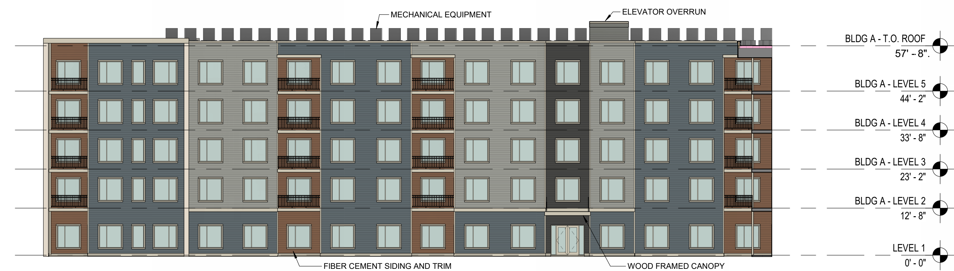
05 BUILDING A ELEVATION - WEST Scale: 1/16" = 1'-0"
