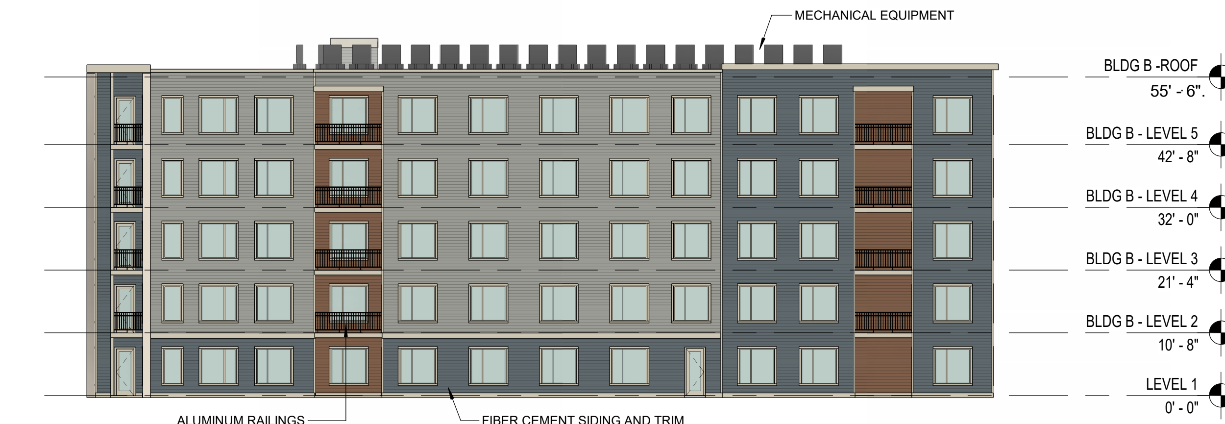
03 BUILDING B ELEVATION - NORTH Scale: 1/16" = 1'-0"
