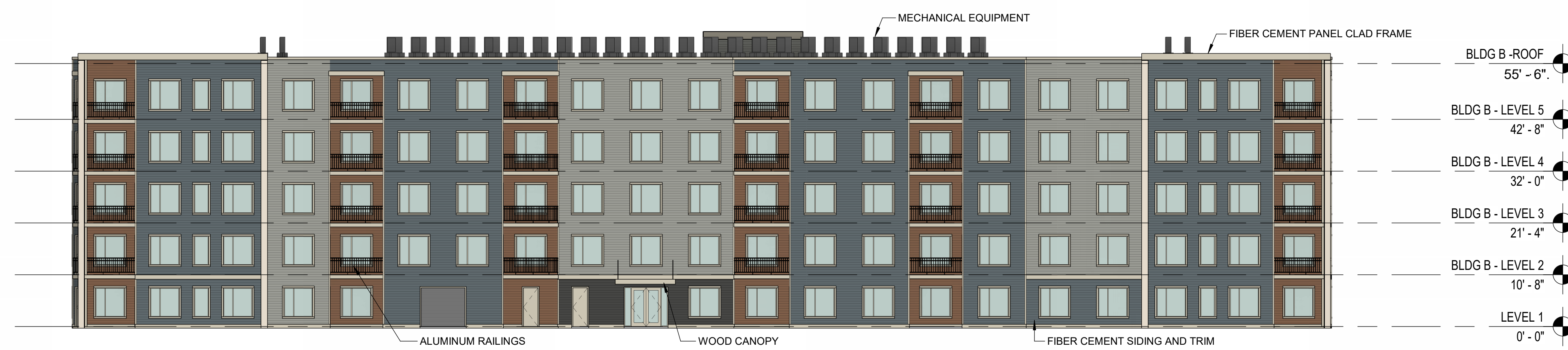
04 BUILDING B ELEVATION - EAST Scale: 1/16" = 1'-0"
