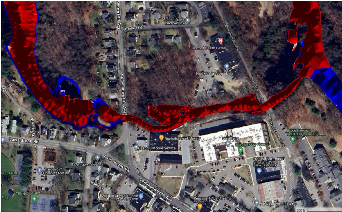
Figure 16. Total Load Capacity Difference During 2yr-24hr Flood Frequency Rising Limb
