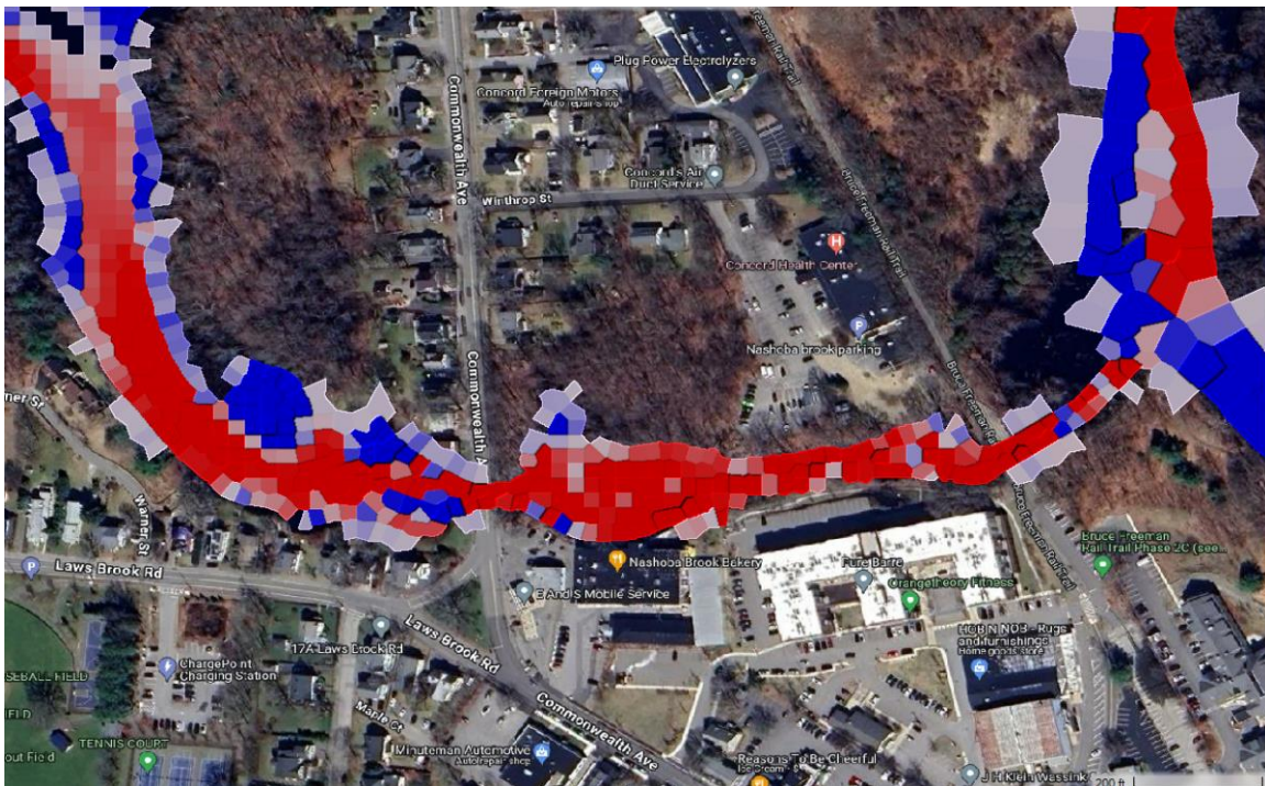
Figure 19. Bed Change for Post Removal Conditions After 2-yr 24-hr Flood Frequency
