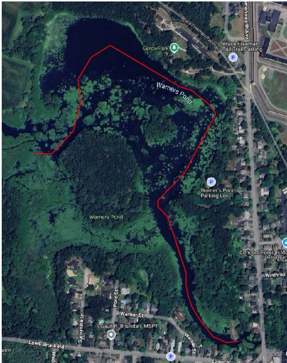
Figure A. Location of channel through Warner's Pond. The approximate channel width and depth were estimated using a profile line drawn in Aterra's HEC-RAS model that follows the deepest sections of terrain.
