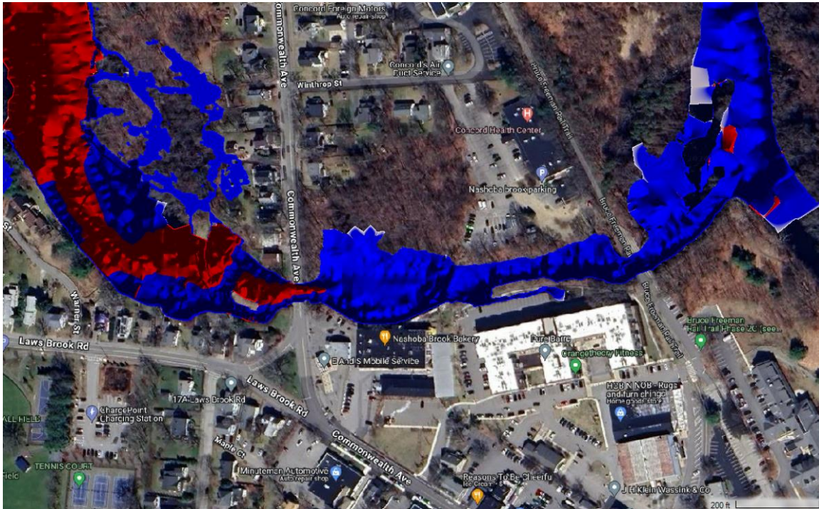
Figure 22. Total Load Capacity Difference During 5-yr 24-hr Flood Frequency Falling Limb
