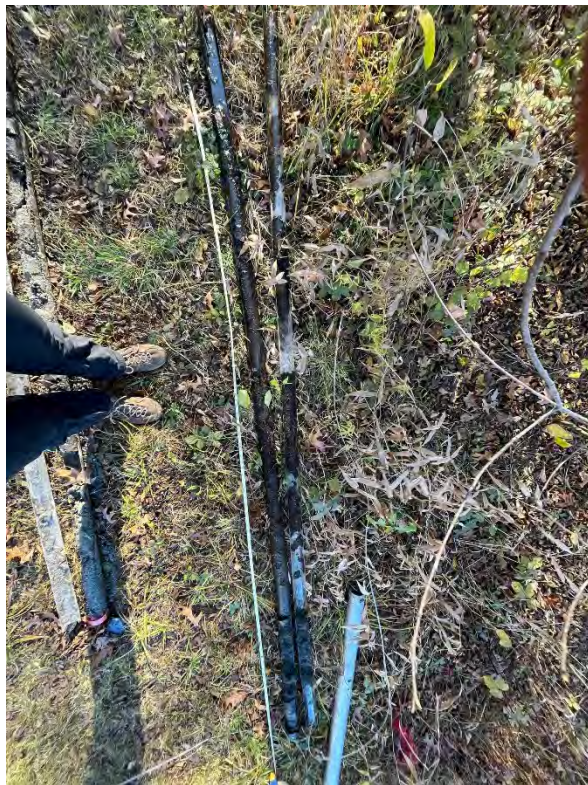
6: SED-02 sediment core sample.
