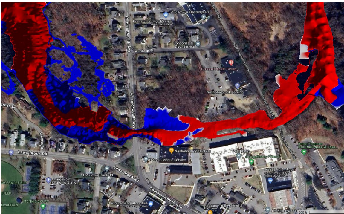
Figure 21. Total Load Capacity Difference During 5-yr 24-hr Flood Frequency Peak
