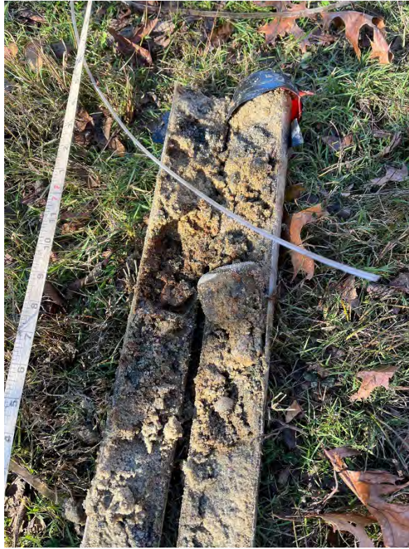
29: SED-05 sediment core sample.
