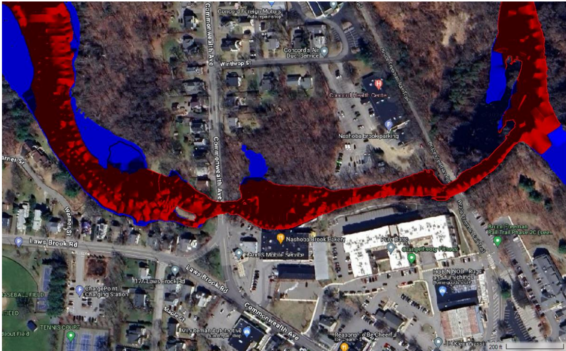
Figure 13. Total Load Transport Capacity Difference During Bank-full Flow
