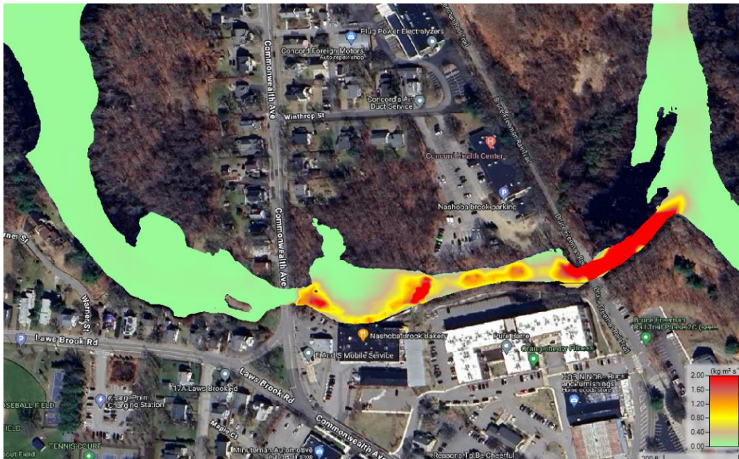
Figure C27. Stream Power Map ( \text{kg m}^2 \text{s}^{-3} ) for Post Removal Conditions During 2yr-24hr Flood Frequency
