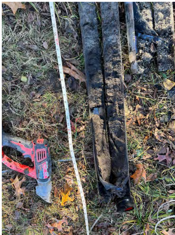
18: SED-03 sediment core sample.
