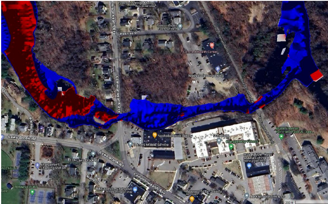
Figure 18. Total Load Capacity Difference During 2-yr 24-hr Flood Frequency Falling Limb
