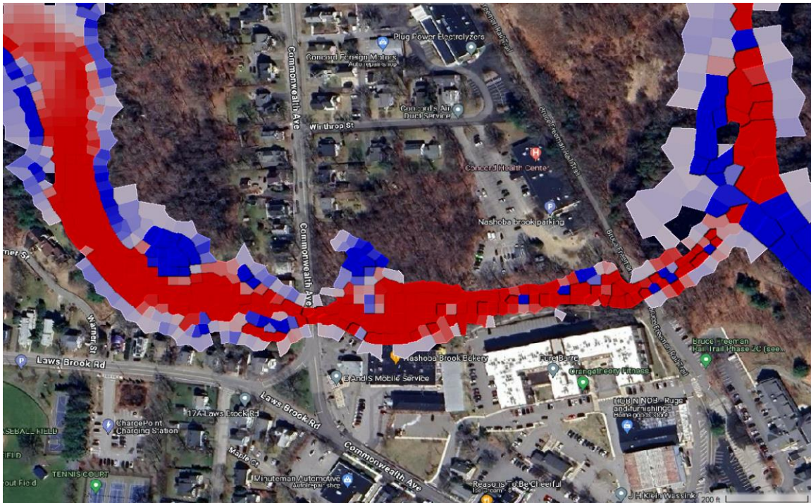
Figure 23. Bed Change for Post Removal Conditions After 5-yr 24-hr Flood Frequency
