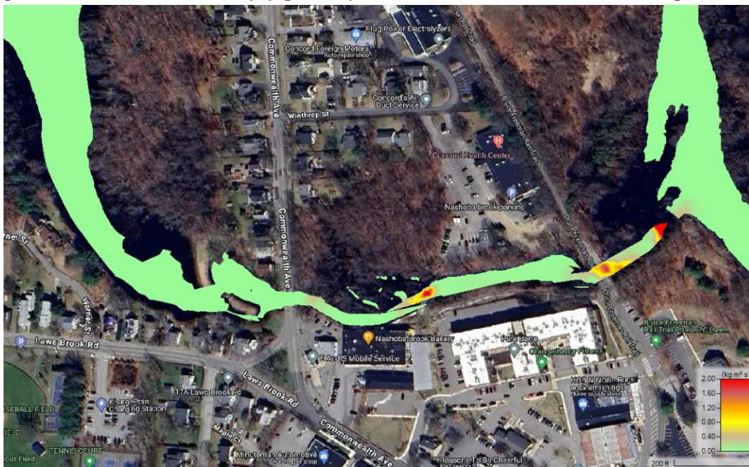
Figure C23. Stream Power Map ( \text{kg m}^2 \text{s}^{-3} ) for Post Removal Conditions During Baseflow
