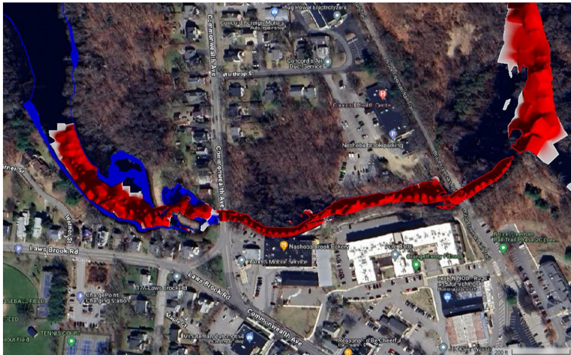
Figure 12. Total Load Transport Capacity Difference During Baseflow
