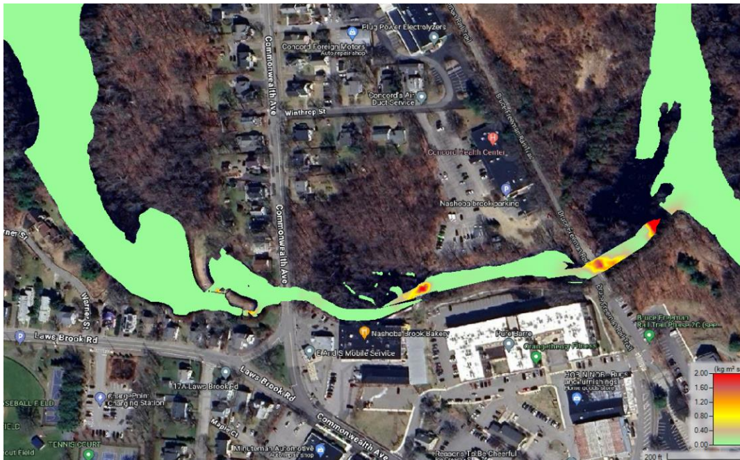
Figure C22. Stream Power Map ( \text{kg m}^2 \text{s}^{-3} ) for Existing Conditions During Baseflow
