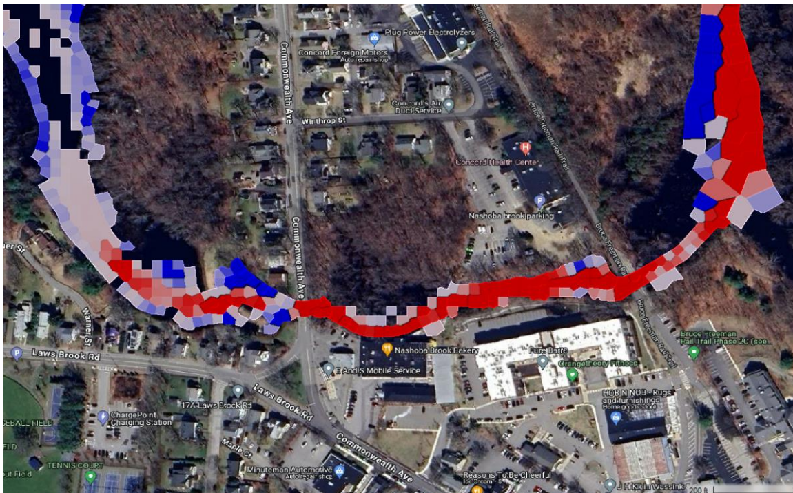
Figure 14. Bed Change for Post Removal Conditions During Baseflow
