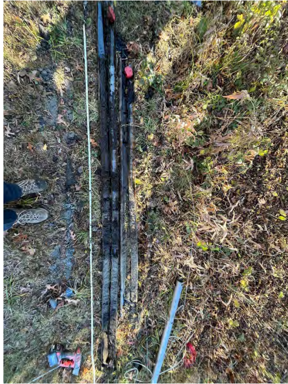
13: SED-03 sediment core sample.
