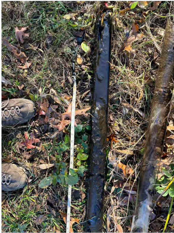
7: SED-02 sediment core sample.
