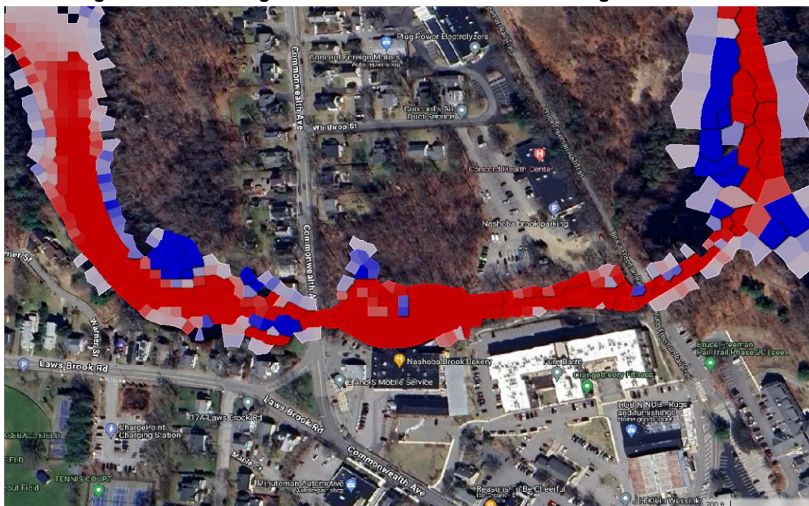
Figure 15. Bed Change for Post Removal Conditions During Bank-full Flow
