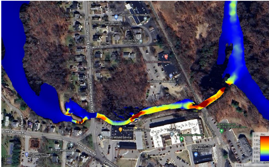
Figure C14. Velocity Map (ft/s) for Existing Conditions During Baseflow
