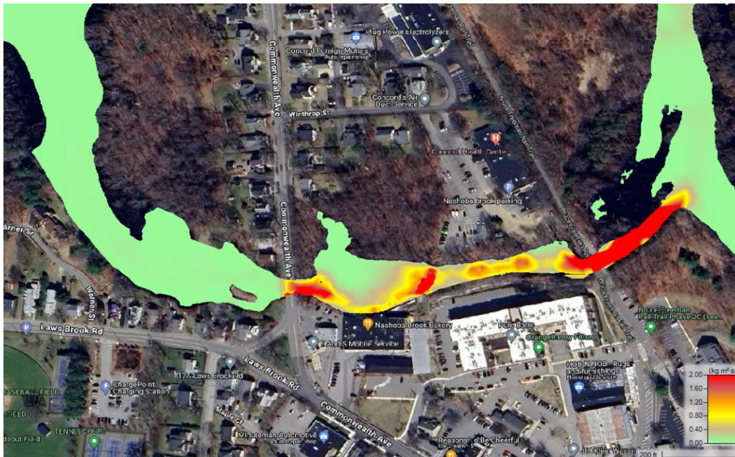
Figure C25. Stream Power Map ( \text{kg m}^2 \text{s}^{-3} ) for Post Removal Conditions During Bank-full Flow
