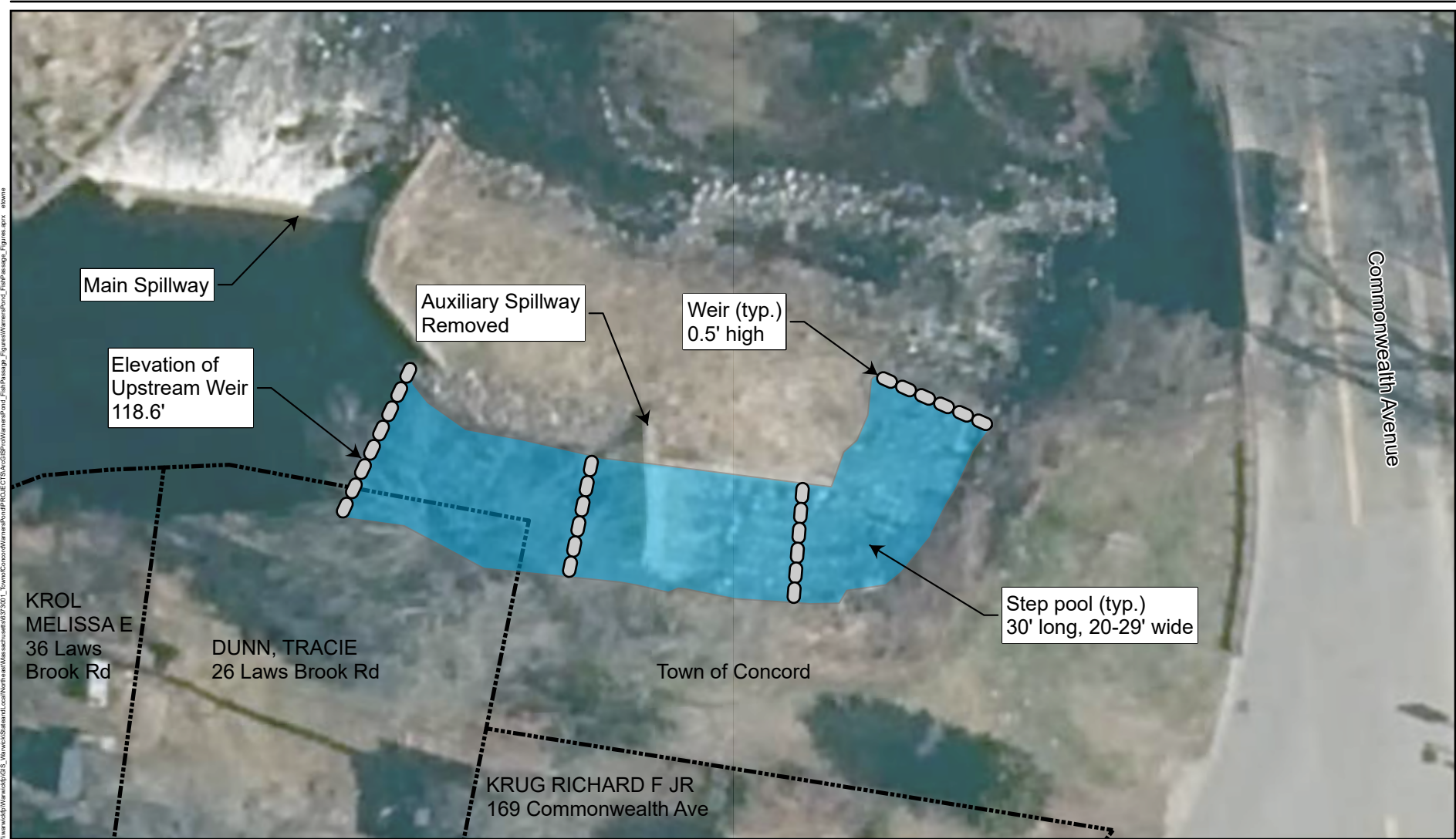
Figure 4 Step-Pool Fishway Conceptual Sketch Warner's Pond Fish Passage Conceptual Feasibility Assessment Concord, MA
