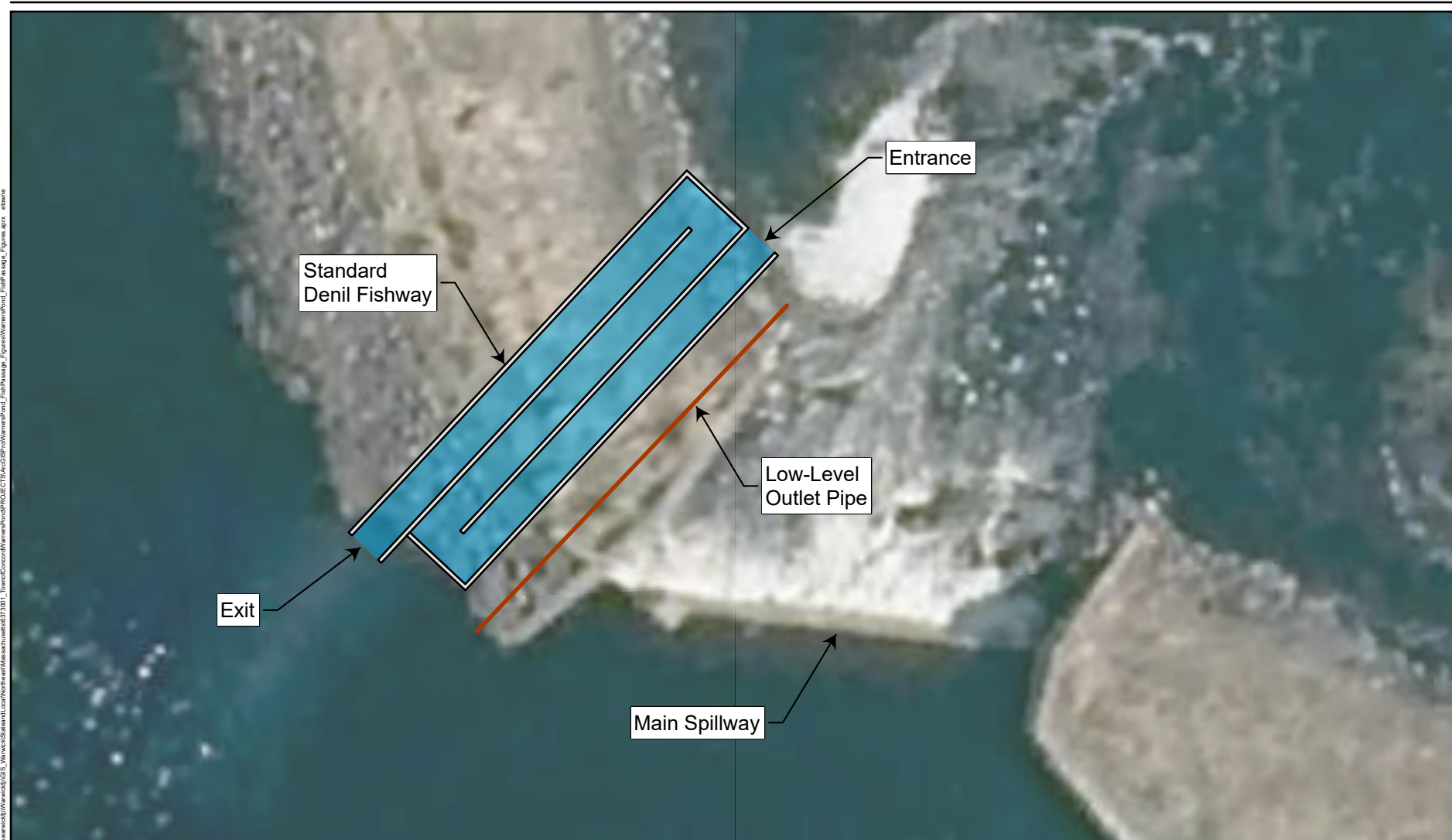
Figure 5 Standard Denil Fishway Conceptual Sketch Warner's Pond Fish Passage Conceptual Feasibility Assessment Concord, MA
